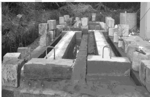
Fig. 3: A Photo of accelerated corrosion of beam specimen
