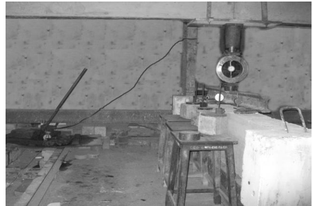
Fig. 6: Position of Dial gauges at centre and load points
